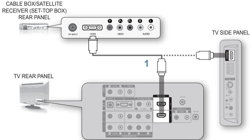
1. Connect an HDMI Cable (Not supplied) between the **HDMI IN (1, 2 or 3)** jack on the TV and the HDMI jack on the Cable Box/Satellite receiver (Set-Top Box).
